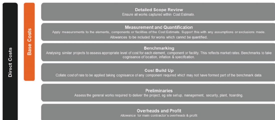
Figure 19 Approach to Cost Estimating, Direct Costs
